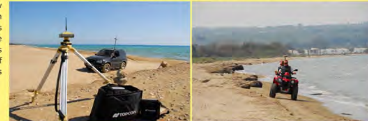
Since walking can waste precious time we also used vehicles on which we set up the Real-Time Kinematic Differential GPS equipment for tracing the present shoreline (2011).
