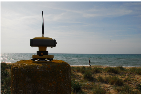
Fig. 4: Using high accurate RTK GPS measurements for the tracing of the present coastline.
