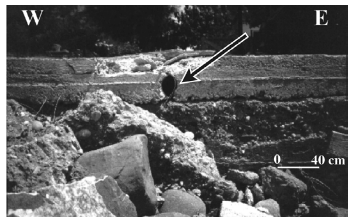
Figure 4 The original circular shape of a PVC pipe deformed to an ellipse.
